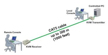
The Kit effectively extends PC KVM (Keyboard, Video and Mouse) control to the Console Receiver and also provides for convenient dual access; in addition to the remote console access, you can also connect a monitor/ keyboard/ mouse set to provide local PC access.
