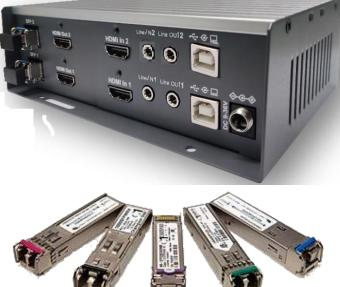
Transmitter then converts back to video, audio, USB... and sends to display, speaker, USB devices. It is a perfect solution for the Central Control Room Dual Head HDMI/DVI KVM applications.
