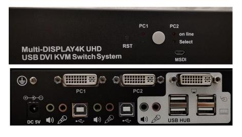
console of a single keyboard, mouse and DVI monitor.
