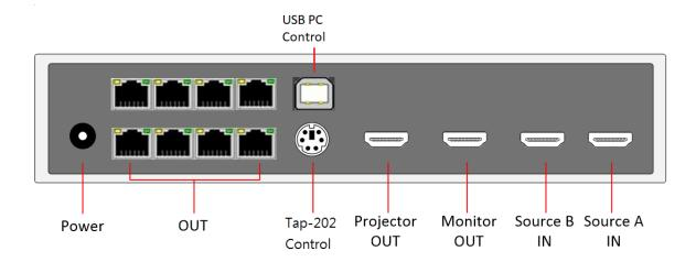
DV-202S 2-User Student box 2 x HD-IN, 2 x HD-Out, 1 x RJ45-In, 2 x RJ45-Out
